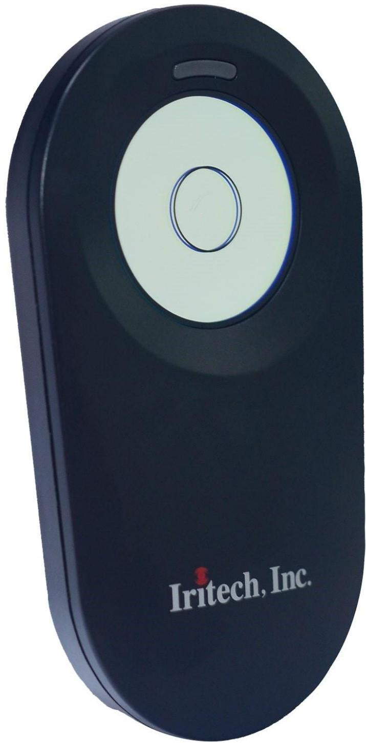
This kind of device works exactly in the same manner as the Fingerprint Recognition device as seen previously. But the only difference is that this is a “non-contactless” kind of technology, in that all the end user has to do is merely point the camera (which is the large circle at the top of the device) in front of their eye at a reasonably close proximity so that a good quality image of the iris can be captured.
